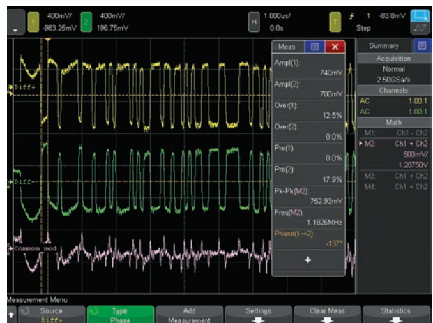
Figure 24. Dual channel WaveGen output of differential arbitrary signals. Common mode is shown as a math function.
