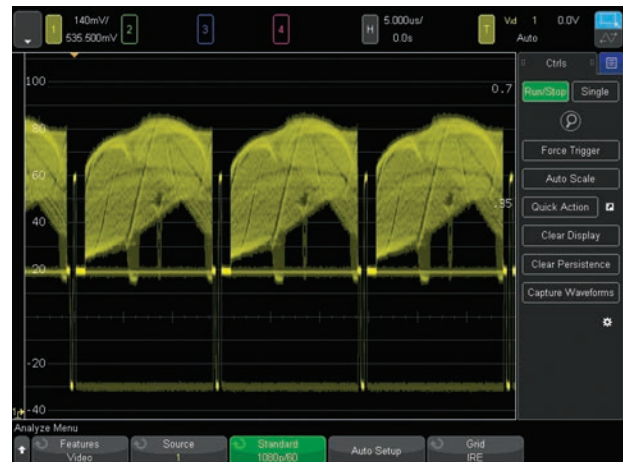
Figure 27. Triggering on 1080p HDTV signal analysis.
