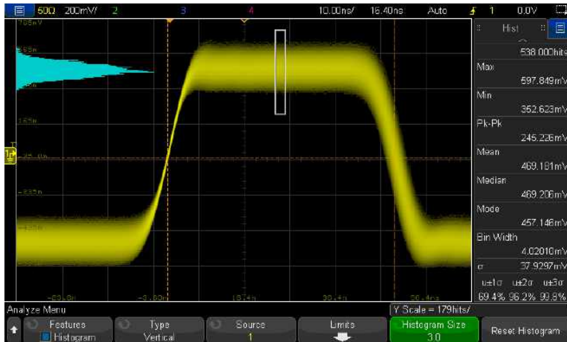
Figure 26. Vertical waveform histogram reveals Gaussian noise with standard deviation of 38 ns.
